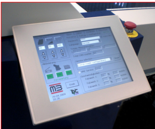
Touch screen display in activated remote control mode of the fully automatic folder prestigeFOLD NET 38.
