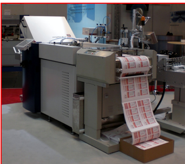
prestigeFOLD NET 52/6 for the production of a two-up selfmailer from the continuous forms stack
